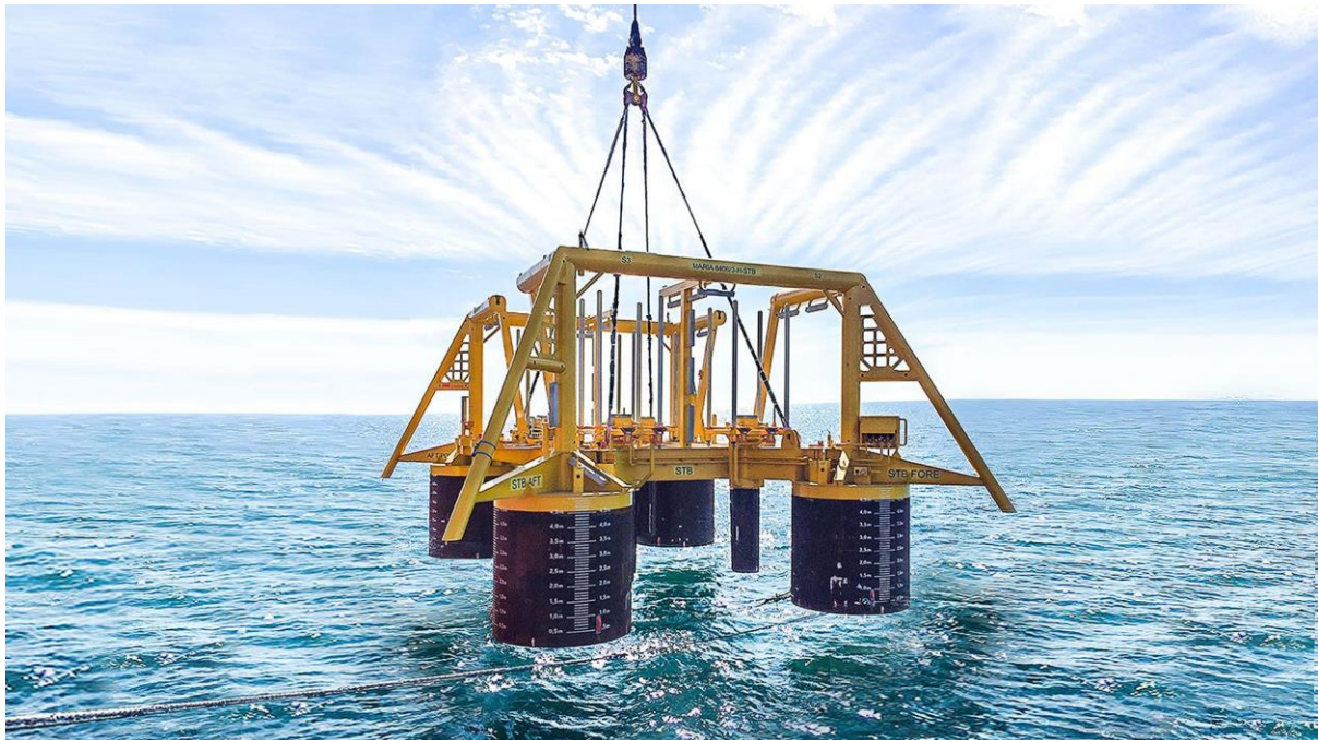
Fig. 1.5. ITS structure for the Maria subsea field in the Norwegian Sea. Adapted from [23]
