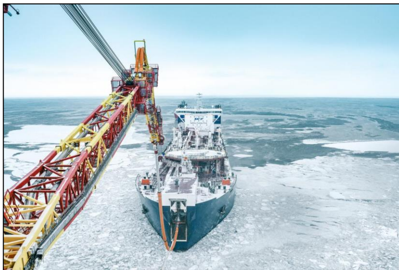
Figure 2.6 – Hydrocarbon offloading from Prirazlomnaya into a tanker [t]
