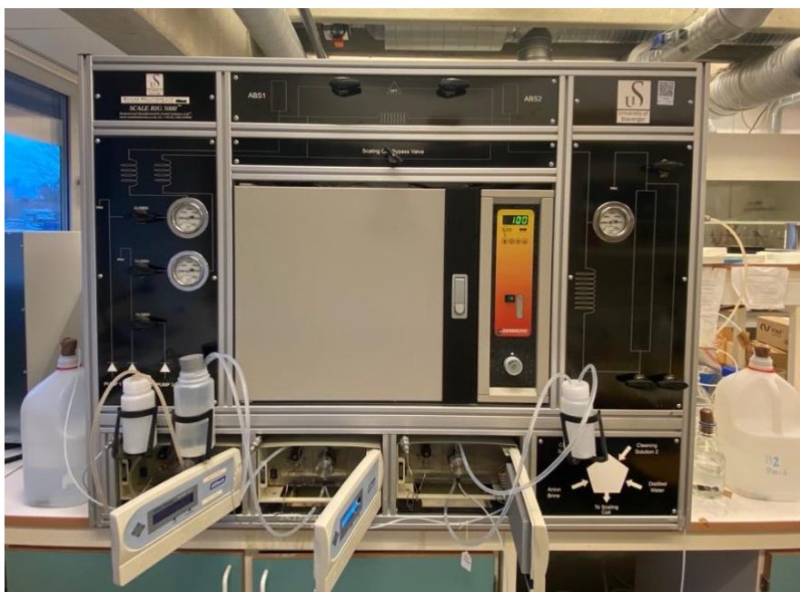
Figure 6: Front view of High-Pressure dynamic tube blocking rig (from left: pump 1, pump 2, pump 3).
