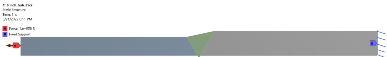
Figure 48 Analysis model boundary conditions - unequal welds between HIP headers and hubs
