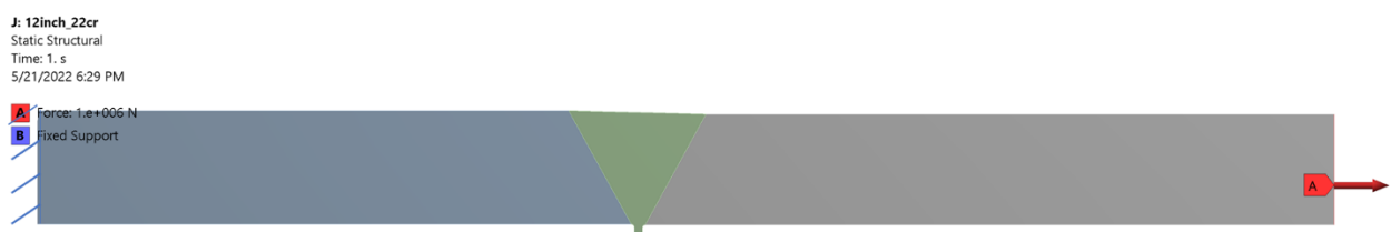
Figure 43 Analysis model boundary conditions - equal welds between HIP headers and hubs
