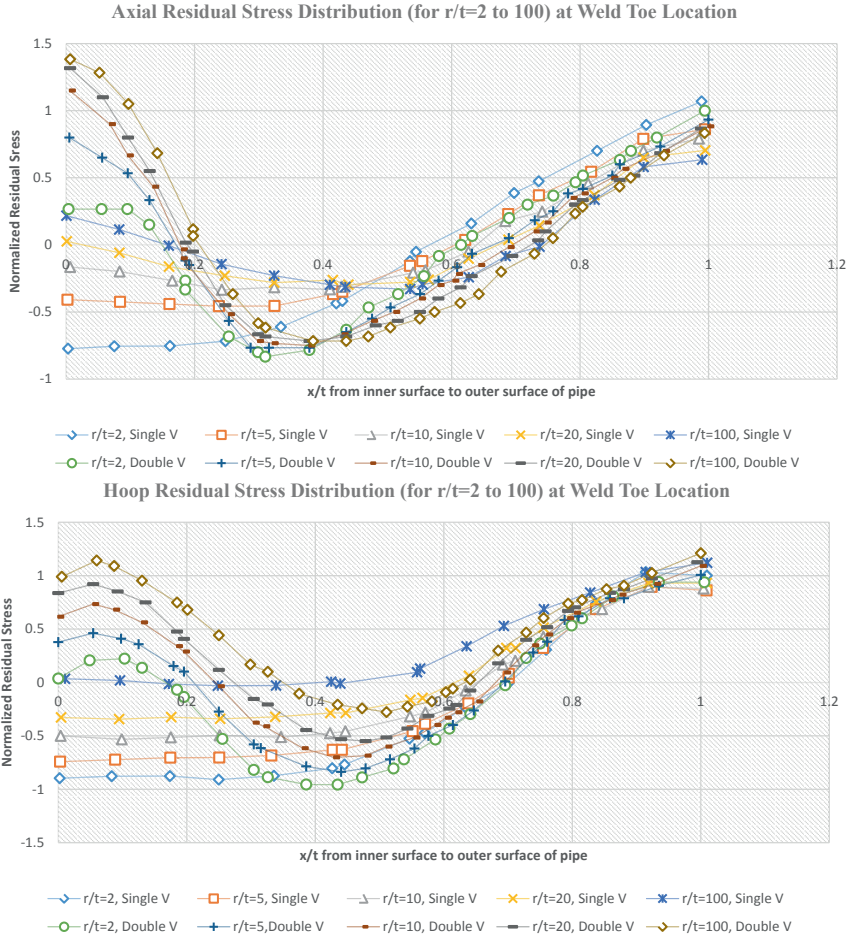
Fig. 8. Residual stress plots ( x/t from inner surface) at weld toe locations for Single V & Double V girth welds with t = 1'' : r/t ratio effects, adapted from [24].
