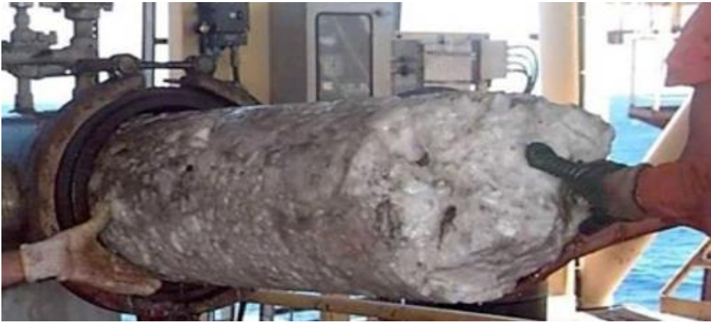
Figure 3.20 Photography picture of hydrate plugging flow line. [51]
