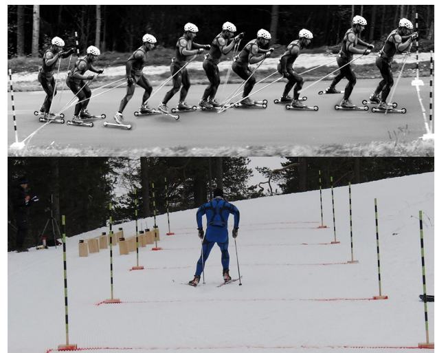
Fig. 1 Upper: One full cycle of the V2 technique. Lower: The 30 m outdoor data-collection area, marked with lines and poles every 7.5 m. Photocells at fixed distances for calculating gliding friction and an anemometer for wind measurement can be seen to the left
