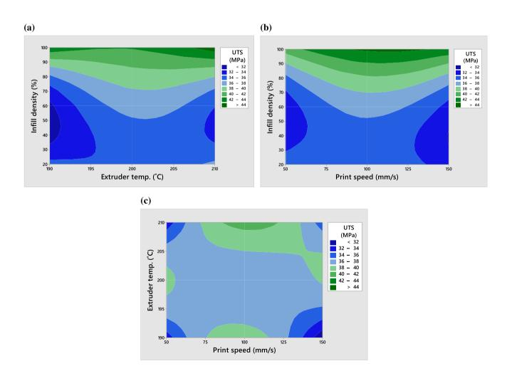
**Fig. 5** Contour plots of **a** infill density (ID) and extruder temperature (ET), **b** infill density and printing speed (PS) and **c** extruder temperature and printing speed with ultimate tensile strength
