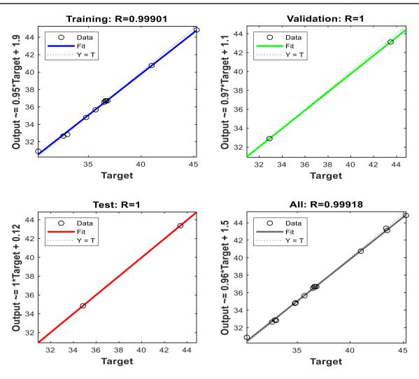
Fig. 6 Regression plots for ultimate tensile strength obtained using artificial neural networks
