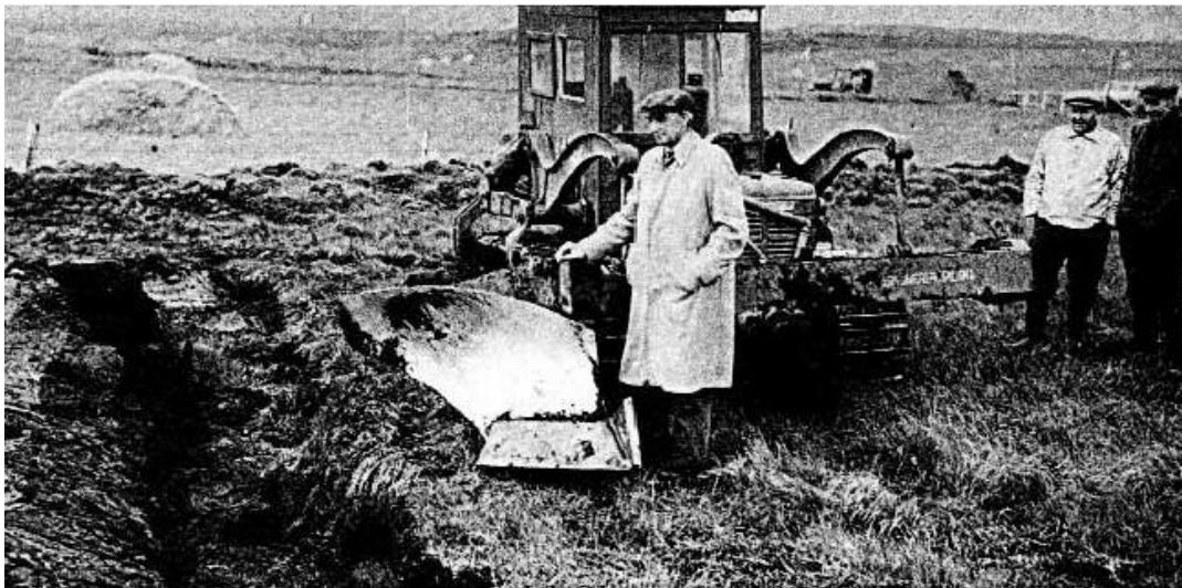
Figure 3. Plowshare made from steel plates of WWII warship Tirpitz. Inventor: R. Skjærpe, an ingenious entrepreneur living in Jæren, Norway. Picture from 1951 [25].
