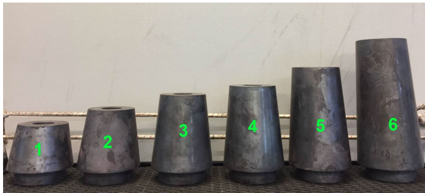
Figure 13. Six cones (part 2) with angles of 10°, 8°, 6°, 5°, 4° and 3° were manufactured. However, only the cone with 3° angle was completely tested in the test.
