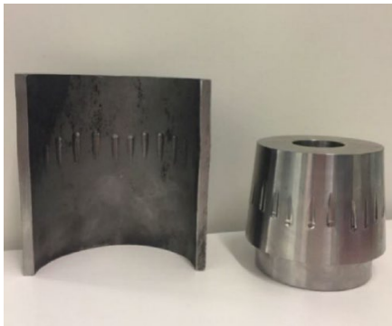
Figure 15. Indentation at the pipe and cone.
