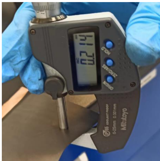
Figure 2.10 Hard carbon electrode with high loading of 25 \text{ mg/cm}^2 .
