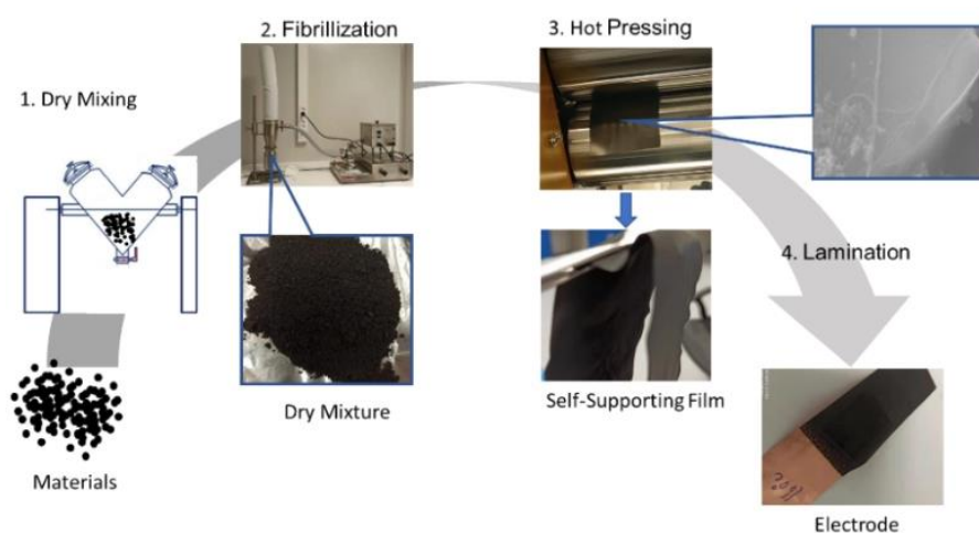
Figure 2.2 Schematic representation of SF anode fabrication procedure.
