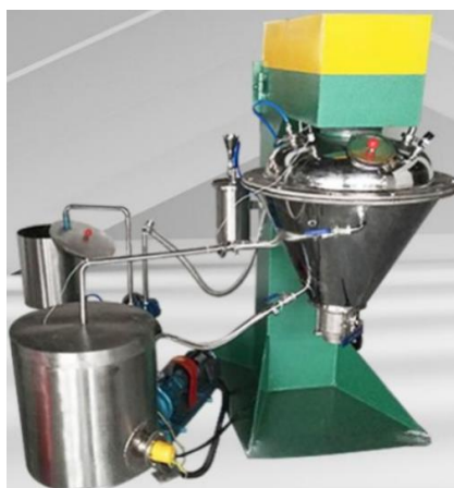
Figure 3.1 The conical mixer with a conical mixing cavity and is equipped with a central rotating shaft, which can rotate at a speed up to 30 m/s.
