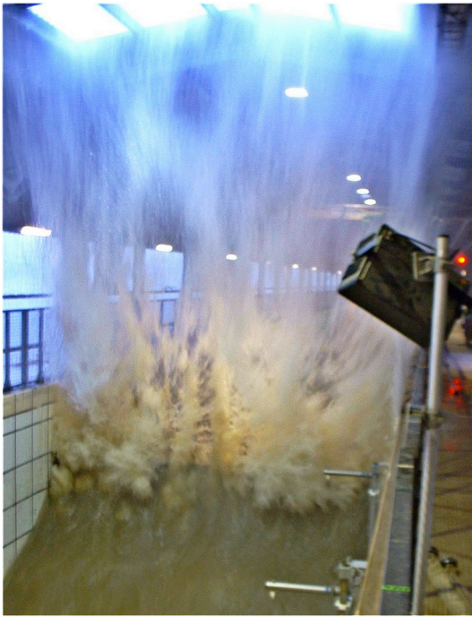
Fig. 34. Air escape from the trapped air pocket in the experiment.
