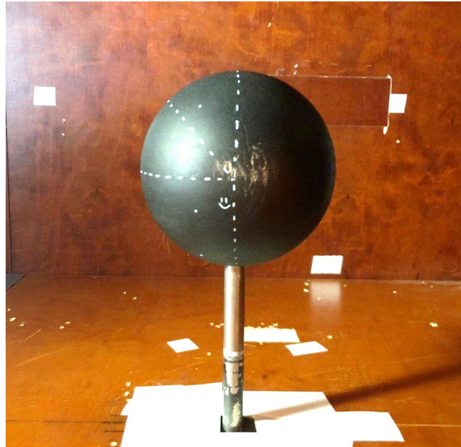
Figure 3. Sphere placed in wind tunnel.
