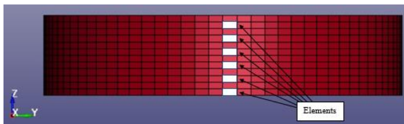
Figure 18. Location of the elements measured for equivalent stress.
