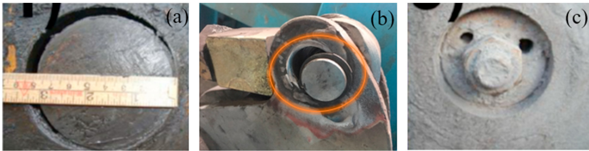
Fig. 5. Std cylindrical pins - (a) and (b) play due to tear and wear of supports, (c) cold welded pin.
