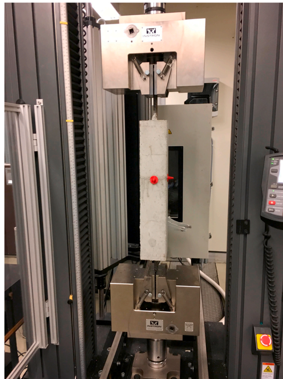
Fig. 3. Loaded RC tie after fixing the surface packers.
