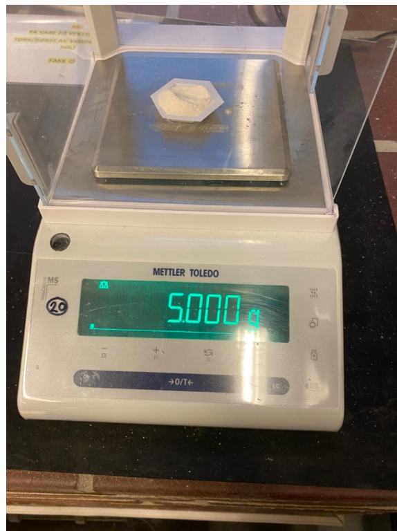
Mettler Toledo weighs 5g PAC to make 1% PAC solution in 5l water.
