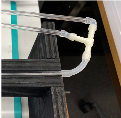
Coupling from test section tube to outlet and differential pressure tube. The setup is not in use at the time photo was taken.
