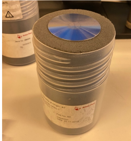
Cone/Plate used with Amplitude sweep test and Hysteresis test.
