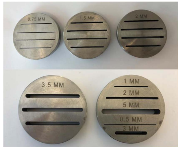
Fig. 1 Slotted steel discs for testing of LCM pills
