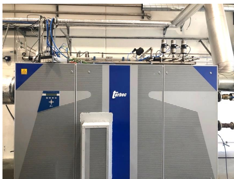
Figure 2. Turbec T100 unit with modified combustor and fuel train for flexible fuel operation.
