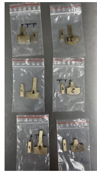
Figure 3.10 Fractured tensile specimens sectioned and ready for SEM examination
