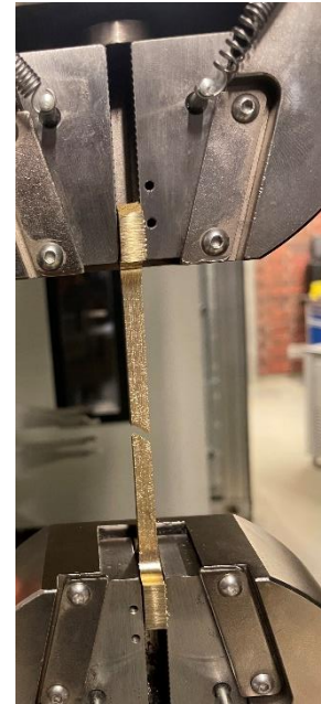
Figure 5.1 TT3 after fracture. The incorrect positioning of the specimen in the grips resulted in the load not to pull uniaxially along the long axis of the specimen.
