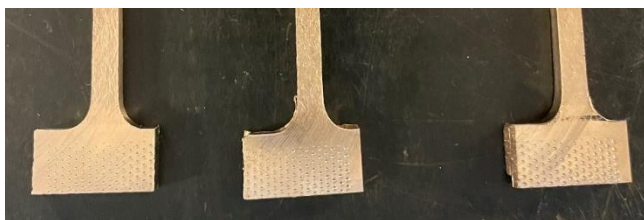
Figure 3.8 The bottom part of the three test specimens TT1, TT2 and TT3 after removing material from the right side of each end, making them ready for testing.
