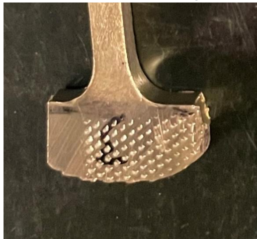
Figure A.8 TT3 placed incorrectly in the testing machine.
