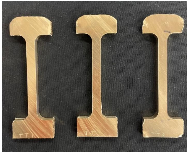
Figure 3.7 The three tensile test specimens TT1, TT2 and TT3 before removing material from one side of each end.
