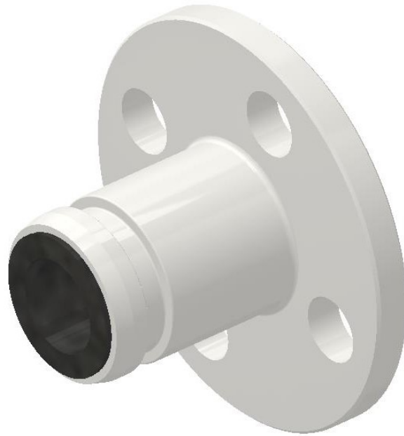
Figure 28: Mounted Iglidur X plain bearing in seal hub made in Inventor
