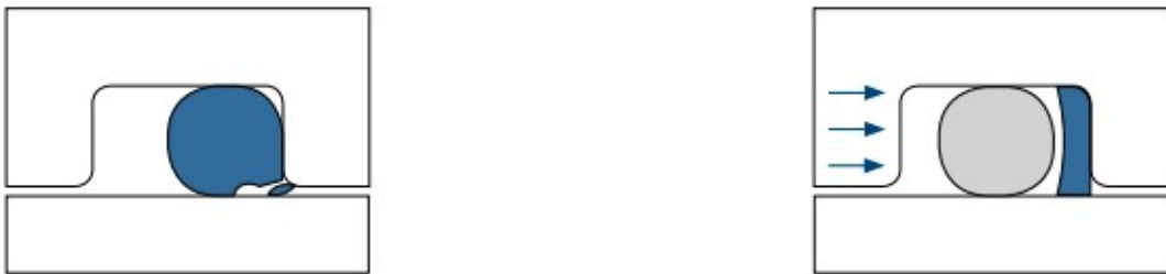
Figure 9: Use of O-ring without back-up ring (left) and with back-up ring (right) [37]
