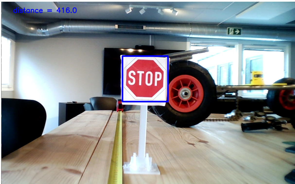
Figure 4.4: An example of the usage of the Stop Sign Detection module to detect a stop sign. The number in the top left corner displays the distance to the stop sign. The measured distance to the stop sign is 416mm.
