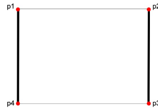
(a) Original image frame in the 3D perspective with the two detected lane lines. (b) Convert to 2D perspective with the four endpoints of the two-lane lines as the frame corners.
