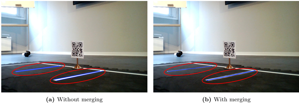
Figure 3.14: Example of merging closed parking lines. In subfigure (a) there are two blue lines in each red oval. In (b) the two lines from (a) are now represented by one line.
