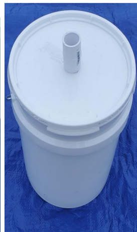
(b) Connection for sample extraction
