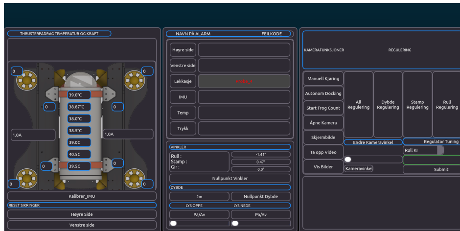
Figure 5.1: Leakage alarm going off in the GUI.
