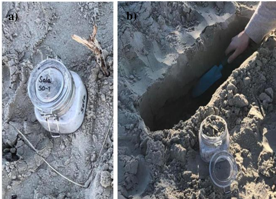
Figure 2 Pictures of the sampling process. a) Surface sample at Sola beach collected in a glass jar. b) Picture showing the sampling of SO-2.
