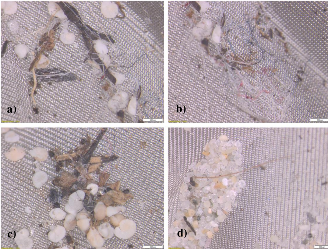
Figure G Optical pictures after separation for surface sample SO-1 a) SO-1 500-250 \mu\text{m} fibers in multiple colors; b) SO-1 500-250 \mu\text{m} several fibers in multiple colors; c) SO-1 500-250 \mu\text{m} transparent fiber, photo credit (University of Milano-Bicocca, Italy n.d.); d) SO-1 500-250 \mu\text{m} red fiber, photo credit (University of Milano-Bicocca, Italy n.d.); e) SO-1 500-250 \mu\text{m} two larger grain probably organic matter with other grains attached, photo credit (University of Milano-Bicocca, Italy n.d.); f) SO-1 250-125 \mu\text{m} interesting light blue particle and a black fiber; g) SO-1 250-125 \mu\text{m} overview of the sample; h) SO-1 250-125 \mu\text{m} overview of the sample; i) SO-1 125-63 \mu\text{m} several white fibers; j) SO-1 125-63 \mu\text{m} black fiber.
