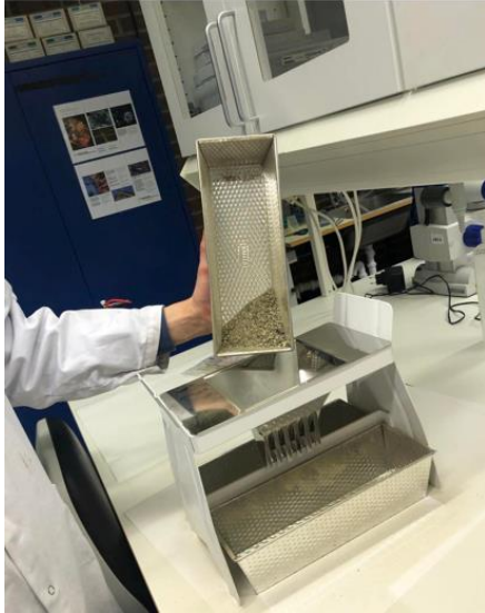
Figure 6 Pictures of the splitting process with the sample splitter to generate two similar samples for further processing.
