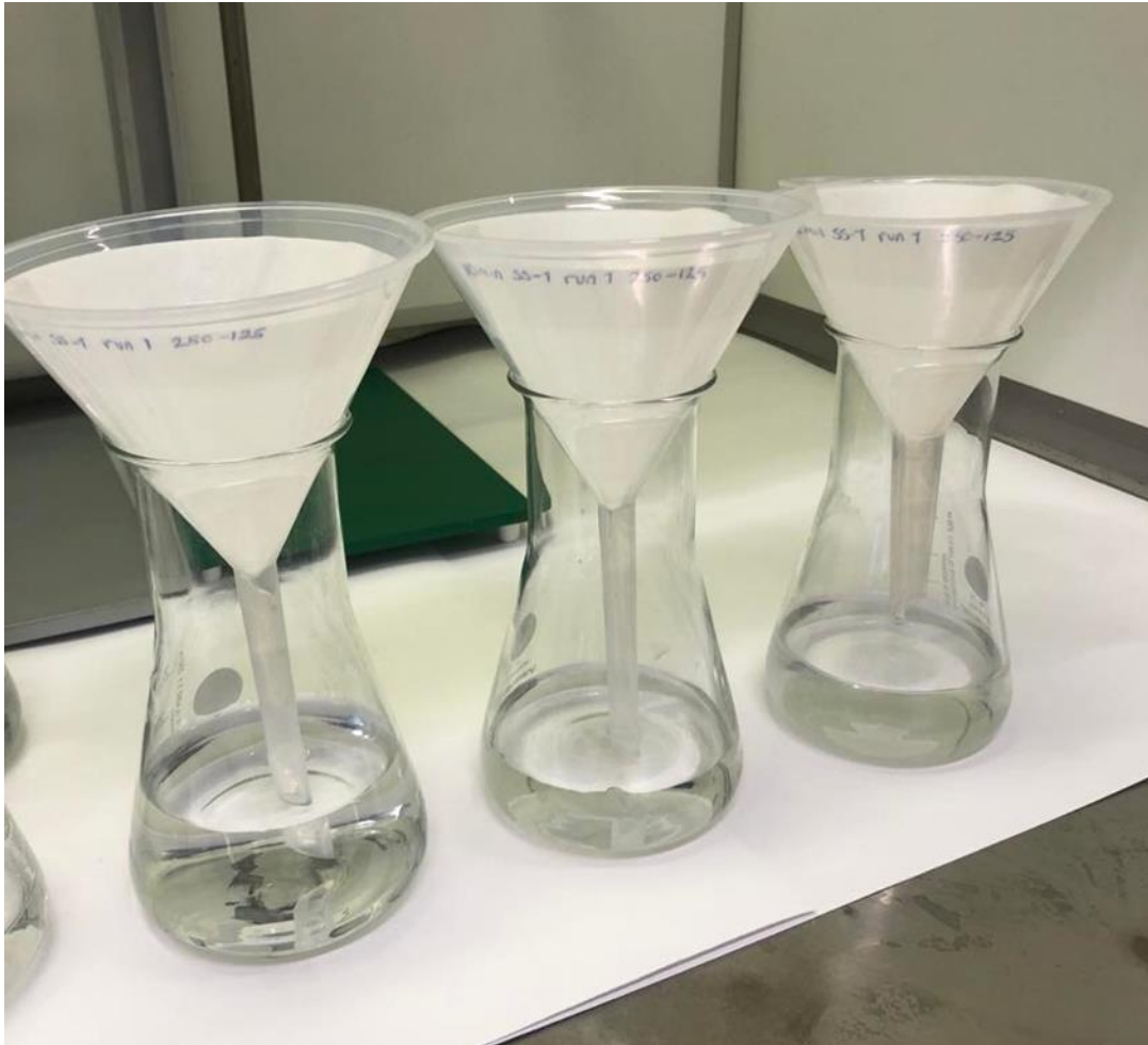
Figure 15 Filtration of the bottom residue.
