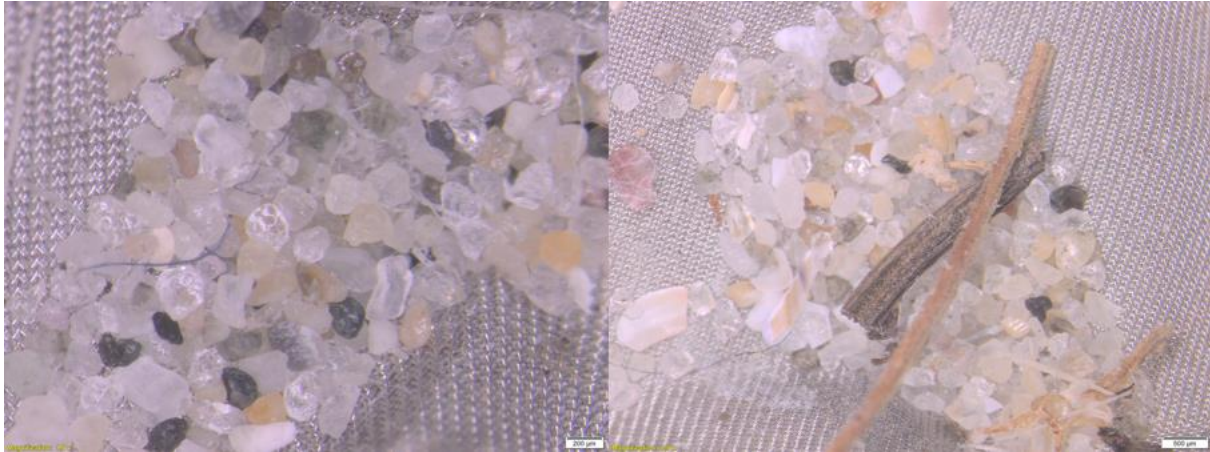
Figure 16 Optical pictures after separation with distilled water. a) BO-1_250-125 \mu\text{m} overview of the collected sample where a blue fiber can be seen; b) SO-1_500-250 \mu\text{m} overview of the collected sample where fibers can be seen.
