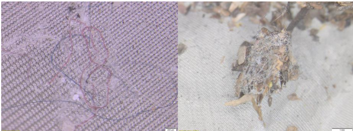
Figure 17 Optical pictures after separation with SPT. a) BO-1_250-125 \mu\text{m} several fibers in multiple colors; b) SO-1_500-250 \mu\text{m} several fibers pushed together into a ball.
