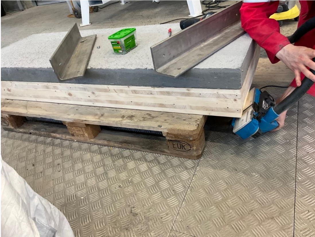
Figure 7.6 Pre-grinding the edges
