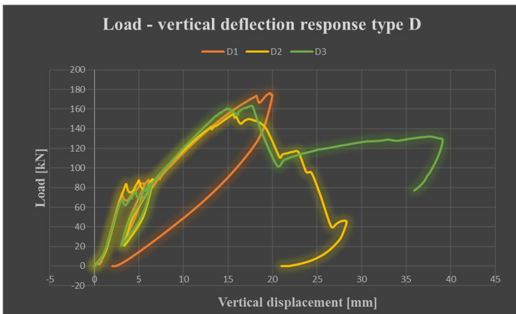
Figure 8.4 Load – vertical deflection response for type D slabs
