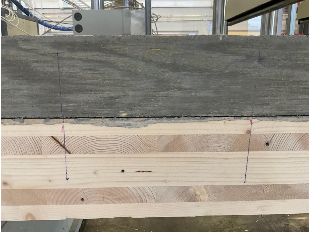
Figure 7.11 Lateral displacement lines on the specimen
