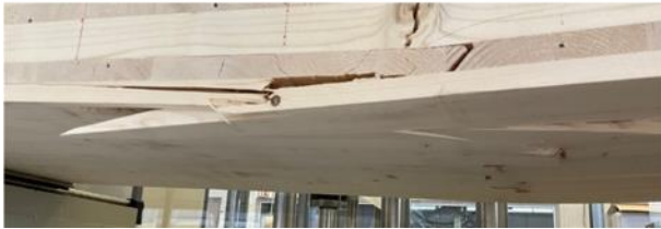
Figure 8.8 Tensile failure underneath the specimens
