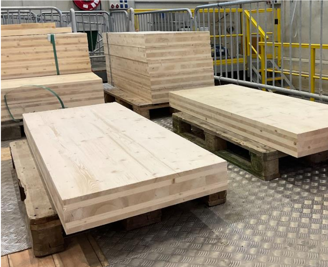
Figure 6.1 15 CLT slabs received
