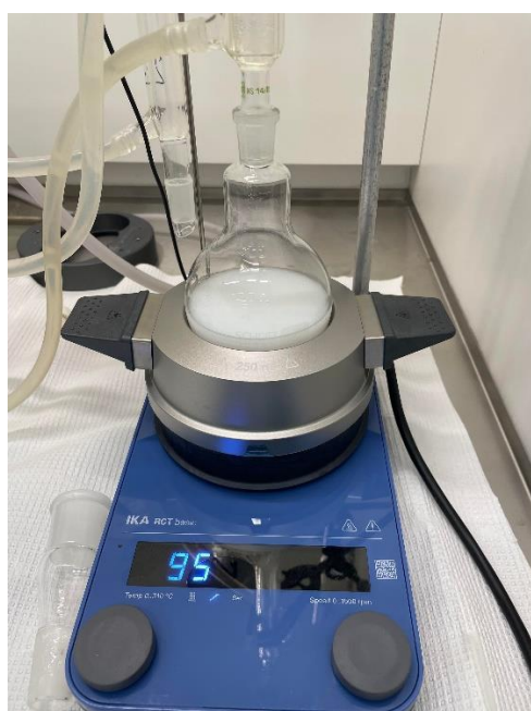
Figure 3-1. Synthesis of Zr-MOF-808-Ac. Experimental setup.
