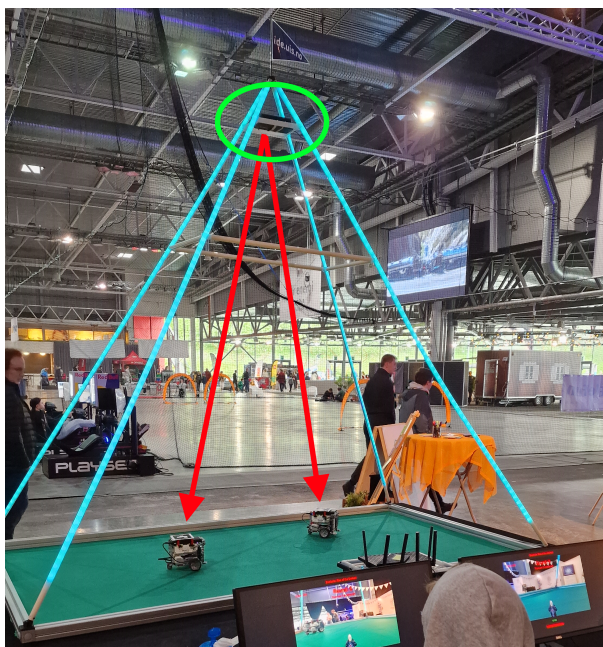
Figure 2.3: The top camera, marked with a green circle, is mounted two meters above the robots. The camera is streaming a continuous video feed which is processed by the server to determine the position and orientation of each robot.
