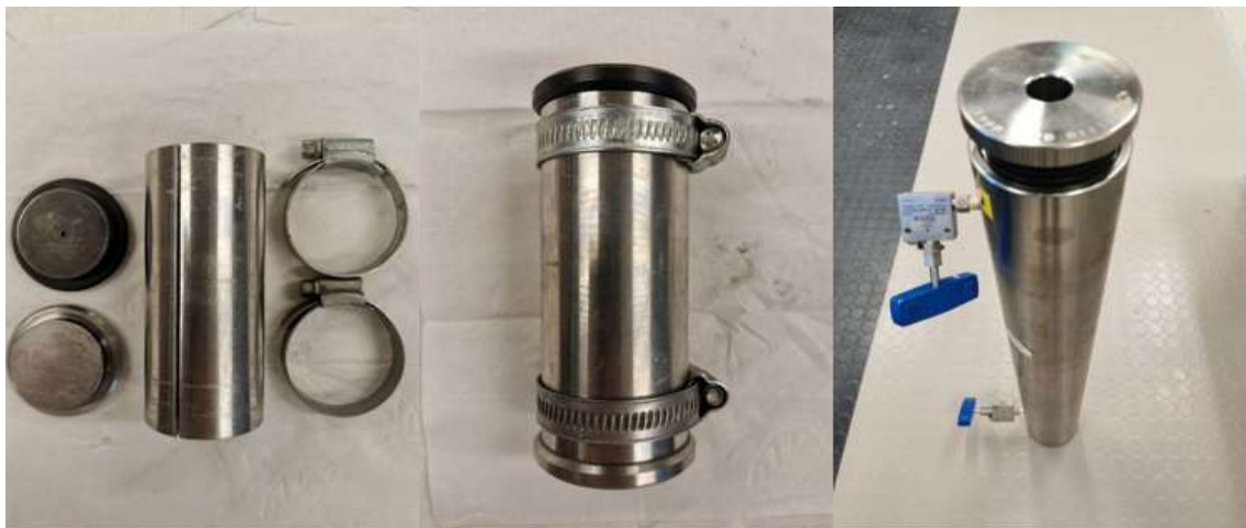
Figure 3: To the left and middle are pictures of a curing mold, and to the right is a picture of an autoclave cell
