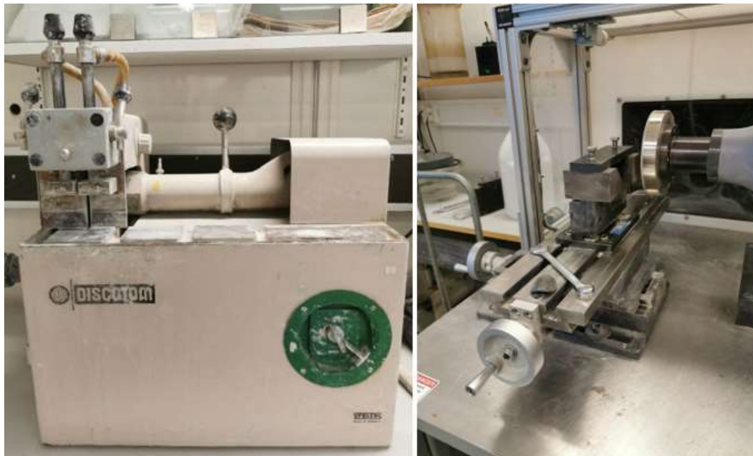
Figure 5: Cutting machine from Discotom to the left and grinding machine from Baldor to the right
