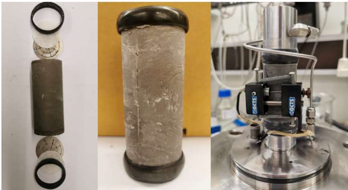
Figure 8: Picture of a core with rubber rings, filter paper, and distributor plates to the left, picture of a core with rubber rings in the middle, and picture of a core installed with extensometer, spiral assembly, and shrinking sleeve to the right.
