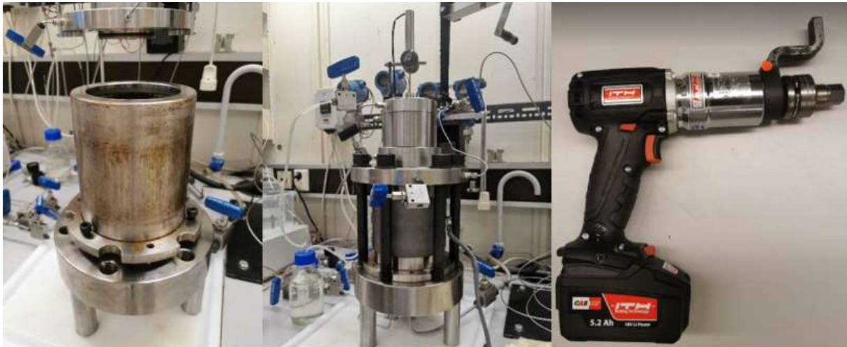
Figure 9: Picture of partly assembled and assembled triaxial cell to the left and in the middle. Electric torque wrench from ITH technologies to the right.
