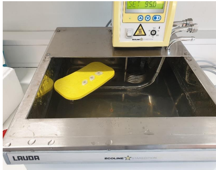
Figure 18: An image of a floating element with tubes containing the bacterial spore suspension fully immersed in a water bath, set at 95°C for the heat treatment experiment. (Picture: Nofima Food Microbiology Lab).
