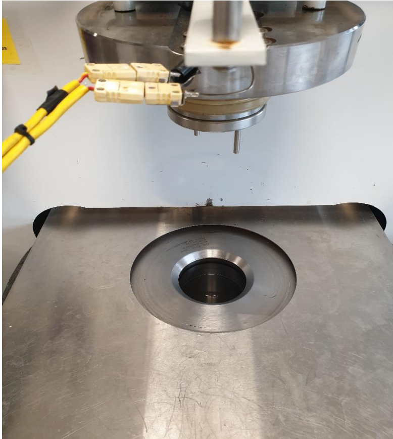
Figure 21: Image of HPP machine showing the loading chamber where sample packages are placed. Picture: NOFIMA Food Processing Laboratory.
