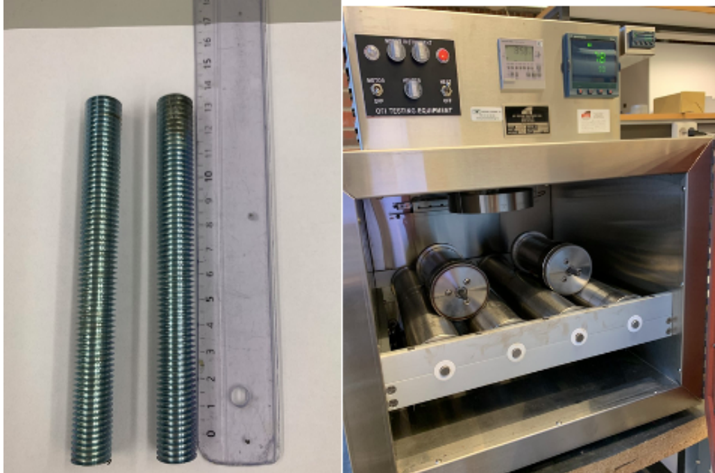
Figure 2.1.3 Threaded steel rod used in Hot Rolling. OFITE Roller Oven 172-00-1-RC
