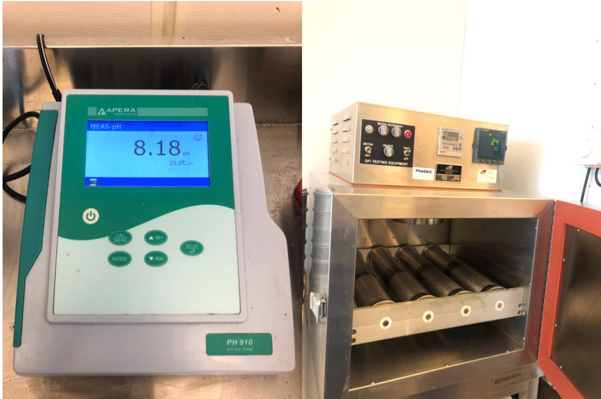
Figure 2: To the left – Apera pH910. To the right - Ofite roller – oven #172-00-1-C.
