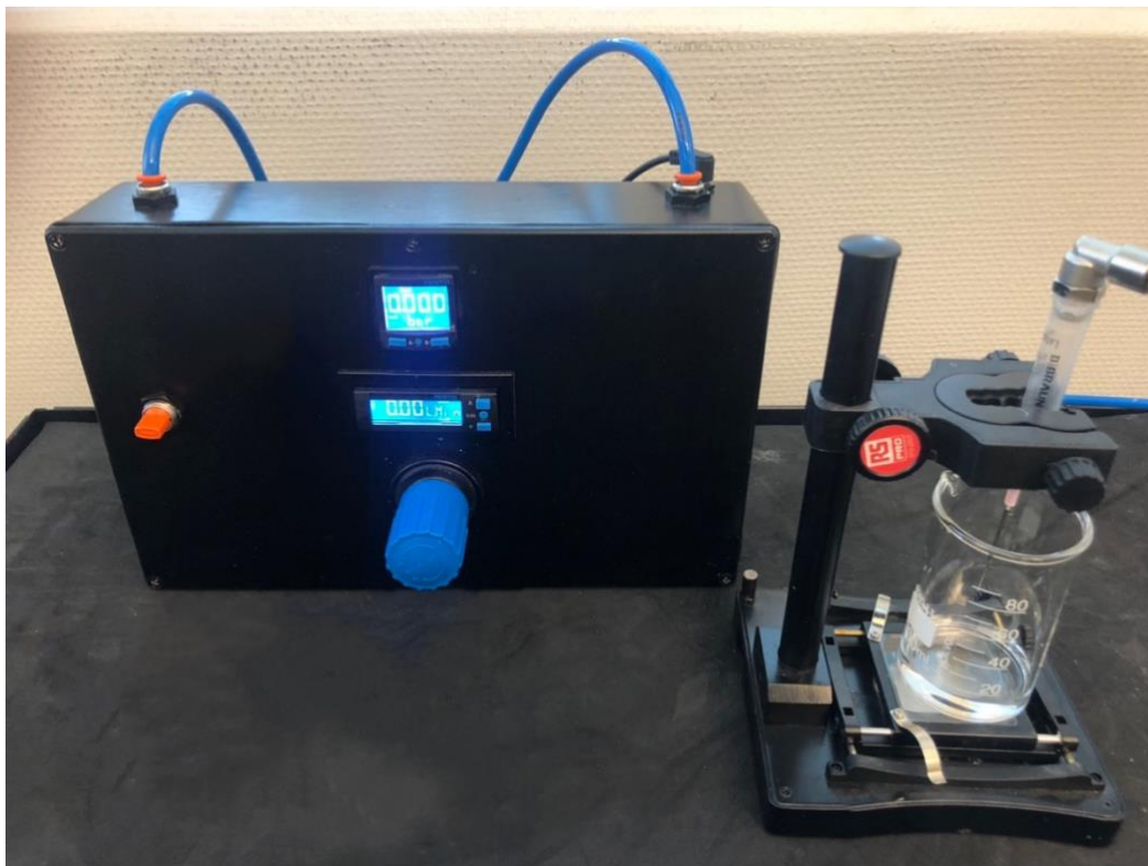
Figure 8: Testing setup - Festo Pressure Regulator LRP-1/4-2.5 and LRP-1/4-0.25, Festo Pressure Sensor SPAN-PO25R and SPAN-P10R, Festo Flowmeter SFAH-10U. B. Braun Omnifix syringe. Needle dimensions (m): Length: 0,046. Diameter: 0,0009
