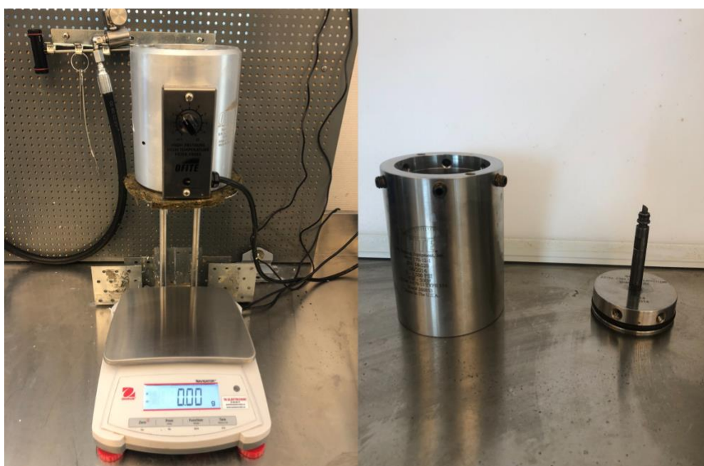
Figure 4: To the left, HTHP Ofite Filter Press Cell. With Ohaus Navigator scale weight located underneath. To the right, Ofite Fluid Cell
