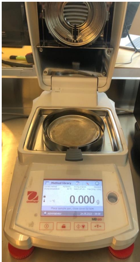
Figure 7: Ohaus MB120 Moisture Analyzer, utilized for moisture removal and conclusion of disc mass.
