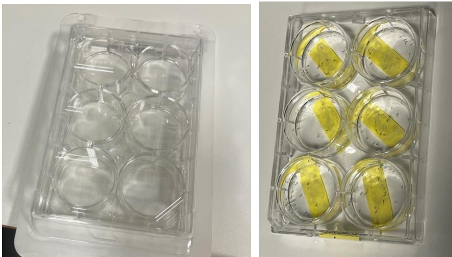
Figure 4: Sterile non-treated 6 wells plate used for the exposure experiment.
