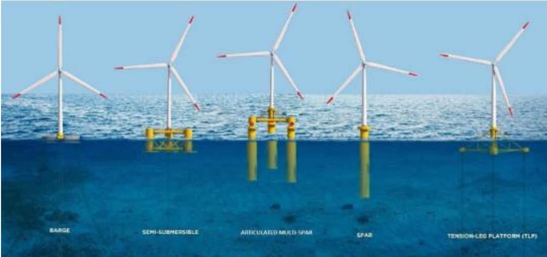
Figure 1: Types of floating foundations.
