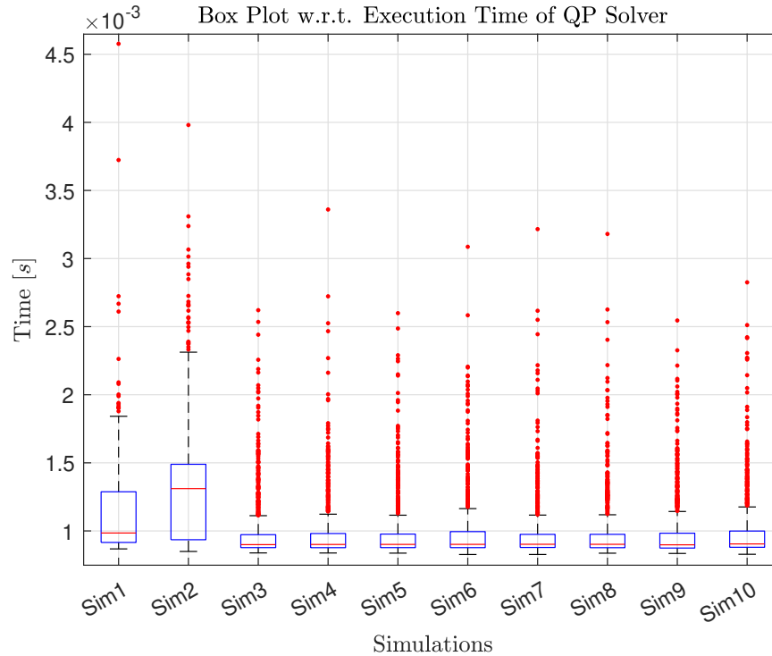
Figure 5.5: Box plot of recorded elapsed time for every 800 QP solver called upon by the linear MPC. Each box represent the data belonging to their respective simulation instance.
