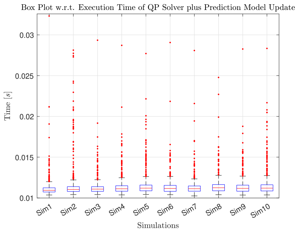
Figure 5.18: Box plot of recorded elapsed time for every 800 control interval (where each control interval consists of one QP solver call, plus one prediction model update) with the adaptive MPC. Each box represent the data belonging to their respective simulation instance.
