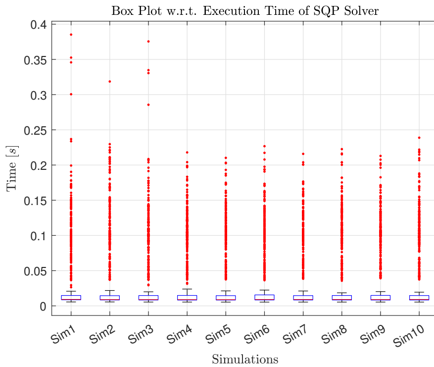
Figure 5.23: Box plot of recorded elapsed time for every 800 SQP solver called upon by the nonlinear MPC. Each box represent the data belonging to their respective simulation instance.
