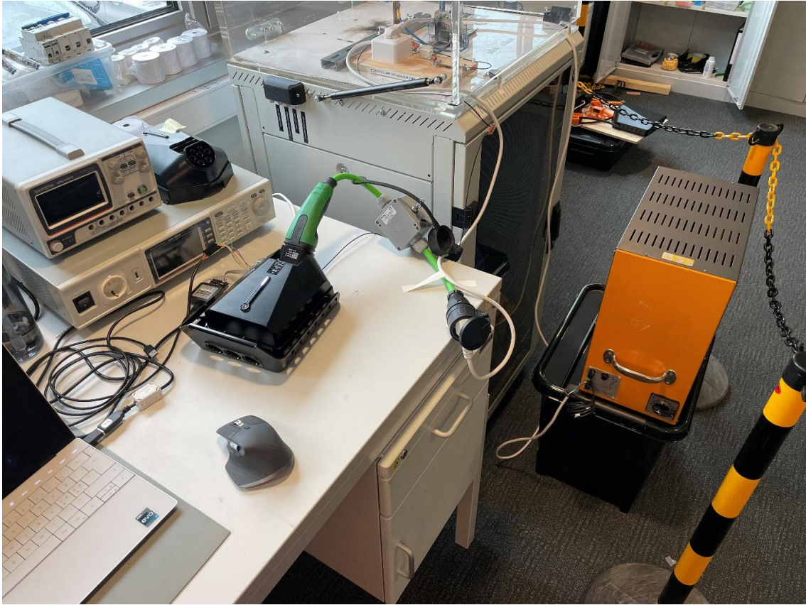
Figure 1: Test setup for data collection using the electric arc generator 2000.
