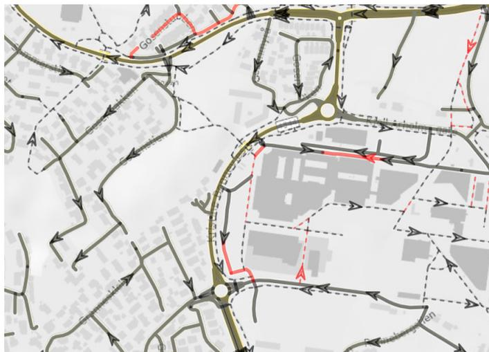
Figure 35: Some "veglenker" highlighted in Vegkart, along with arrows indicating their direction
