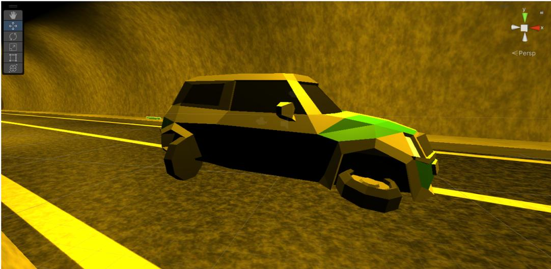
Figure 24: Wheel Meshes incorrectly rotated
