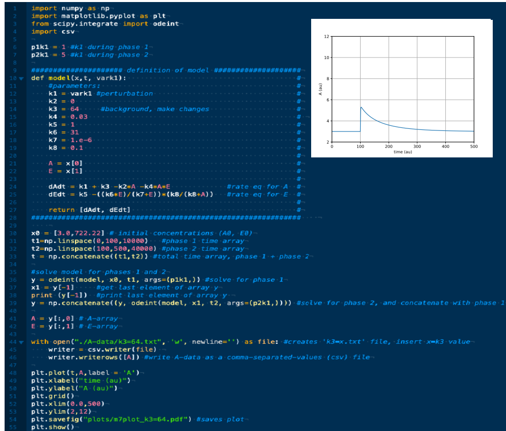
FIGURE A.15: Python script for generating m7's response amplitude of A at background k_3=64 . Making some changes (see above) gives the response amplitude for k_3=4 (see upper right corner). Run this script at k_3=0, 1, 2, 4, 8, 16, 32, 64 . Insert the corresponding initial concentrations of A and E from Fig. 3.6b.
