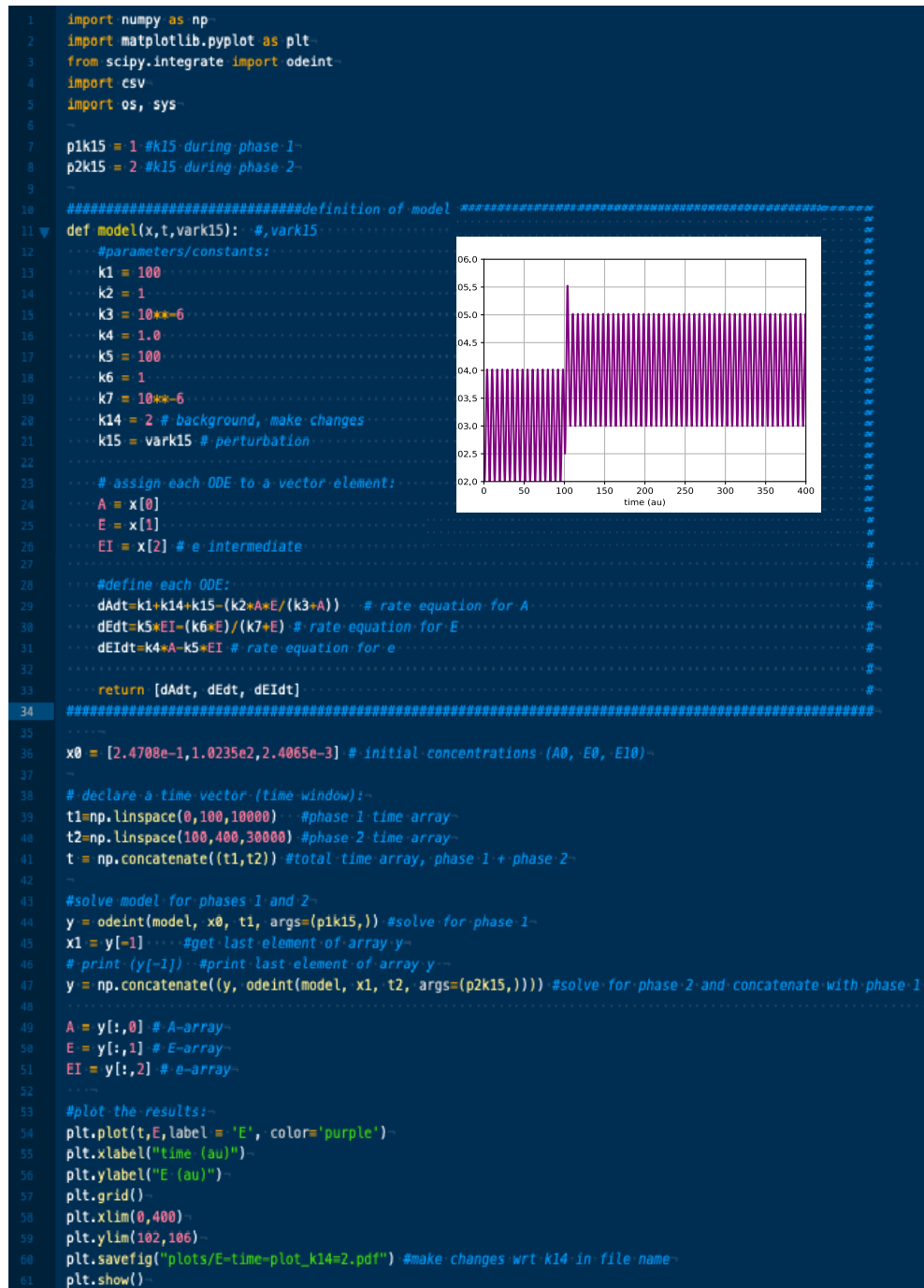
FIGURE A.36: Frequency independent oscillator at k_{14}=0 and k_{15} from 1→2. E is plotted as a function of time.
