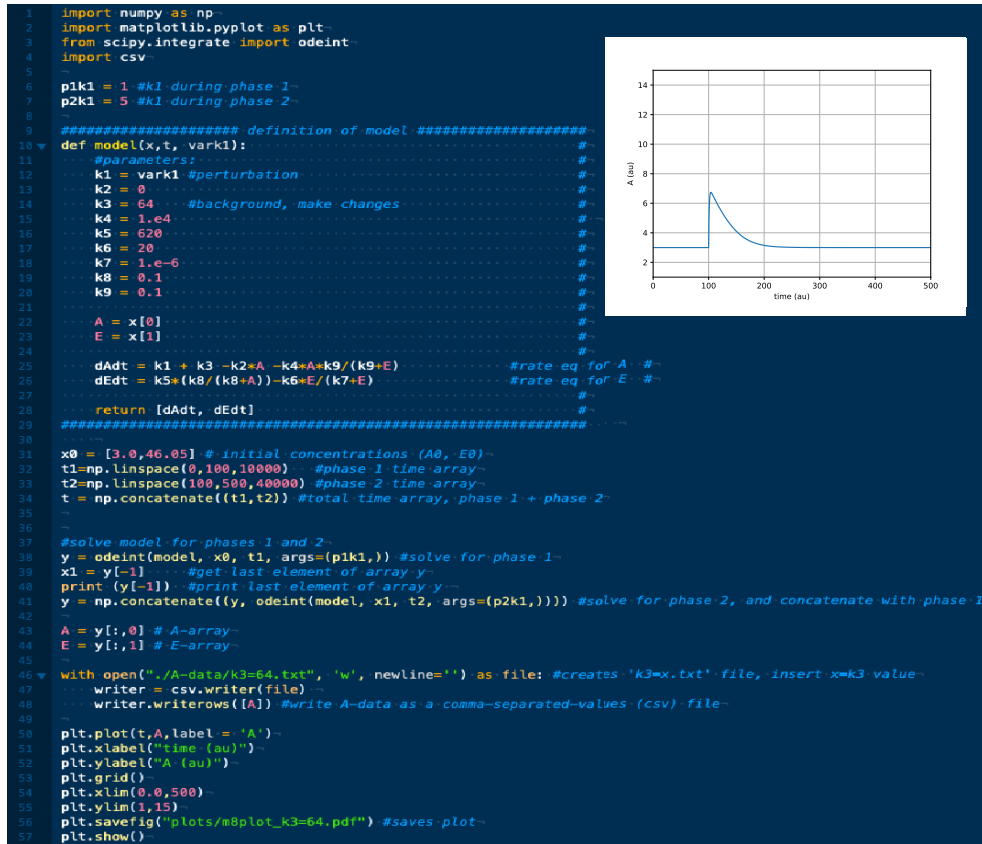
FIGURE A.17: Python script for generating m8's response amplitude of A at background k_3=64 . Making some changes (see above) gives the response amplitude for k_3=2 (see upper right corner). Run this script at k_3=0, 1, 2, 4, 8, 16, 32, 64 . Insert the corresponding initial concentrations of A and E from Fig. 3.11b.
