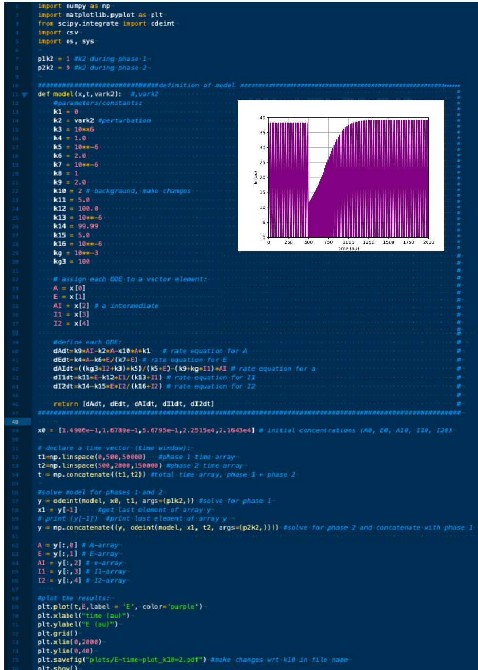
FIGURE A.32: Frequency compensated oscillator with incoherent feedback at k_{10}=2 and k_2 from 1→9. E is plotted as a function of time.
