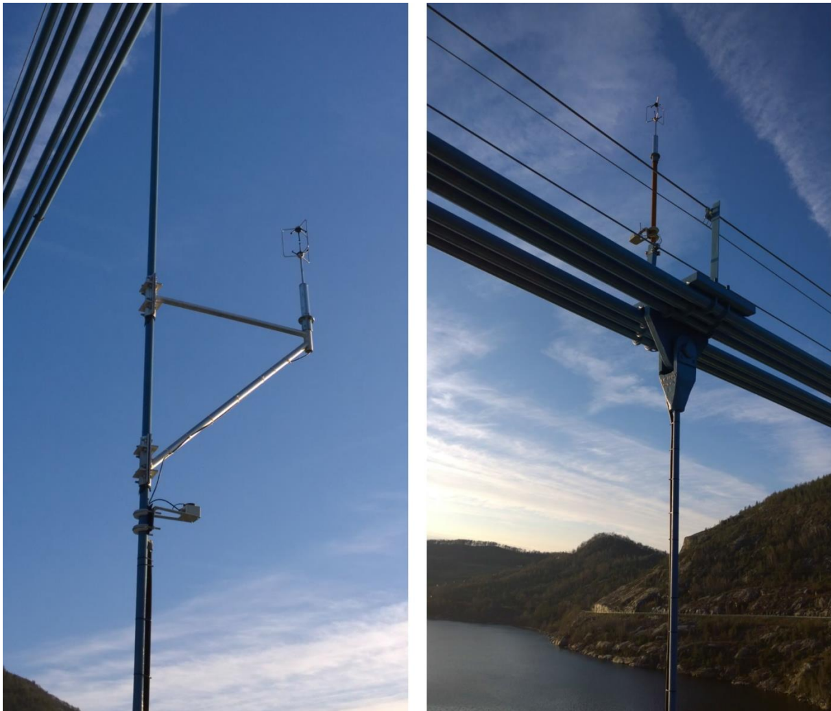
Figure 20: Anemometer mounting positions on a hanger (left) and on a pole on top of the main cable (right) [7, p. 5]
