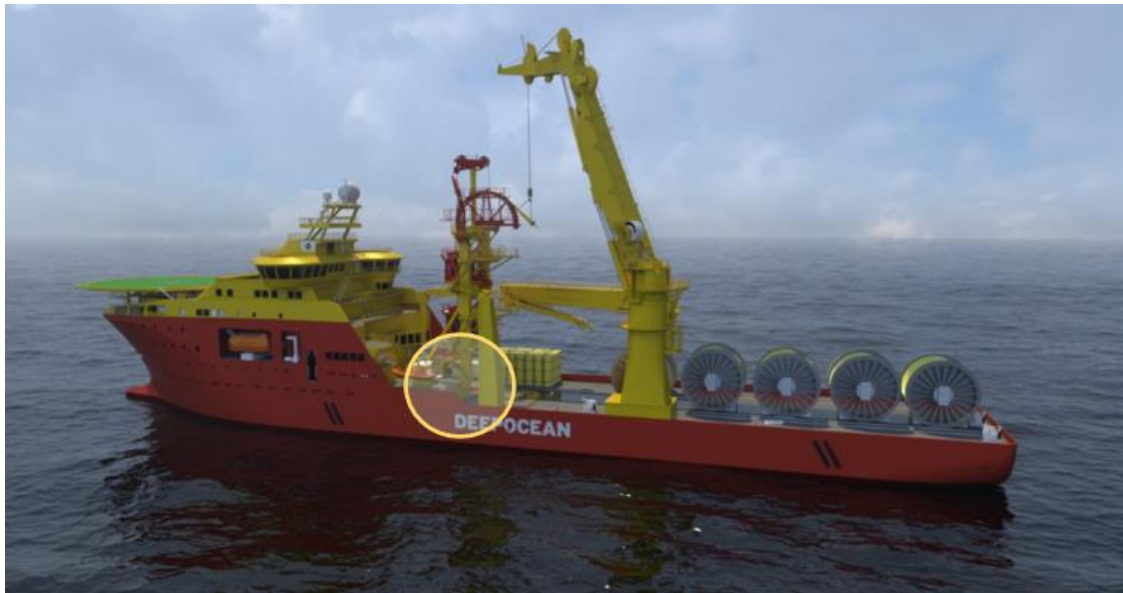
Figure 27: The yellow circle indicates the location of the lower tensioner on Edda Freya's VLS tower [22]
