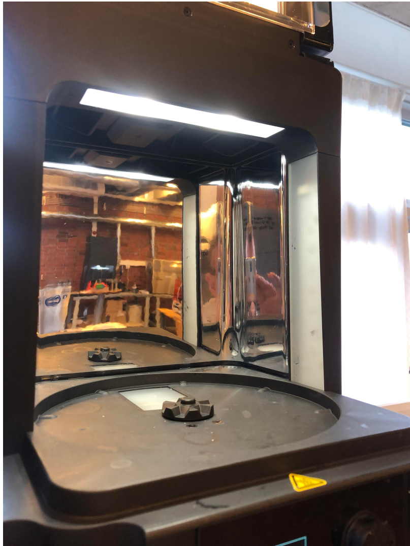
Figure 18: UV Curing chamber internal
