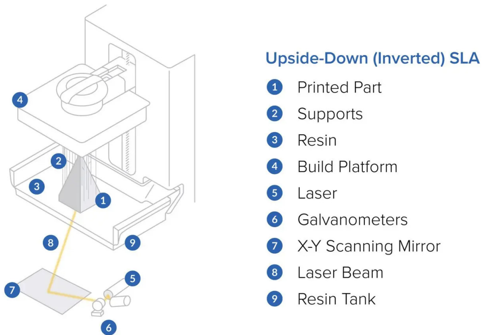
Figure 3: SLA 3D printing schematic illustration (Formlabs, 2023e)
