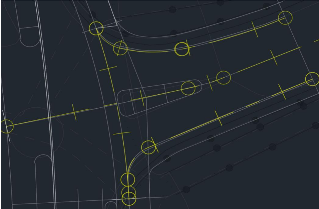
Figure 43 Location of boundary lines for T – intersection
