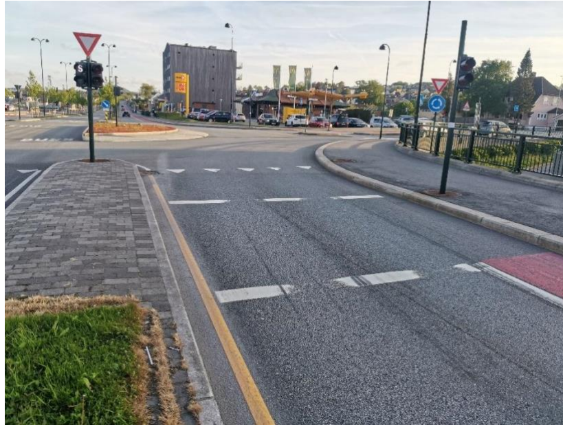
Figure 14 Bike box on bus prioritized roundabout in Mariero (authors picture)
