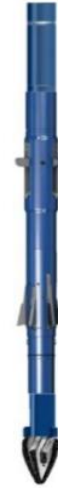
Figure 3.12 A combined tool that both mills the casing and under-reams the formation [18]
