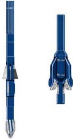
Figure 3.11 Historical section milling performed with two separate tools [18]
