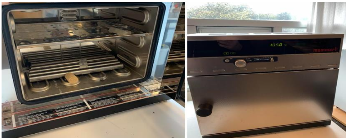
Figure 5.5 Oven used to store samples during heat cycles of approximately 105°C
