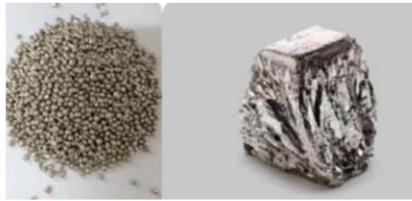
Figure 4.3 Pellet and solid bismuth [35]
