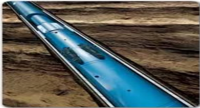
Figure 3.6 Sketch of the Harpoon cut-and-pull spear recovering the casing string [16]
