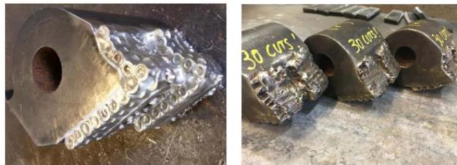
Figure 3.3 New knives (left) versus used knives after 30 cuts (middle) [13]
