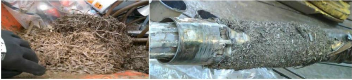
Figure 3.13 Accumulates of Swarf on the tools, forming “bird-nests” [17]
