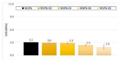
Fig. 3 The effect of chemical admixture C on 1-day UCS
