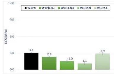
Fig. 5 The effect of NaOH and KOH pellets on 1-day UCS
