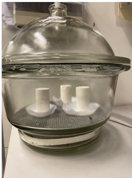
Figure 3.9 Desiccator used for slow drying the cores until target weight was reached
