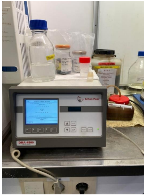
Figure 3.4 Anton Paar DMA 4500 density meter used for density measurement
