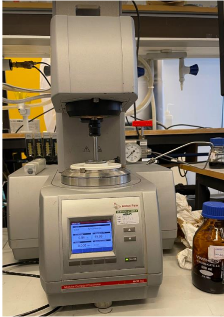
Figure 3.5 Anton Paar MCR 302 rheometer used for viscosity measurements
