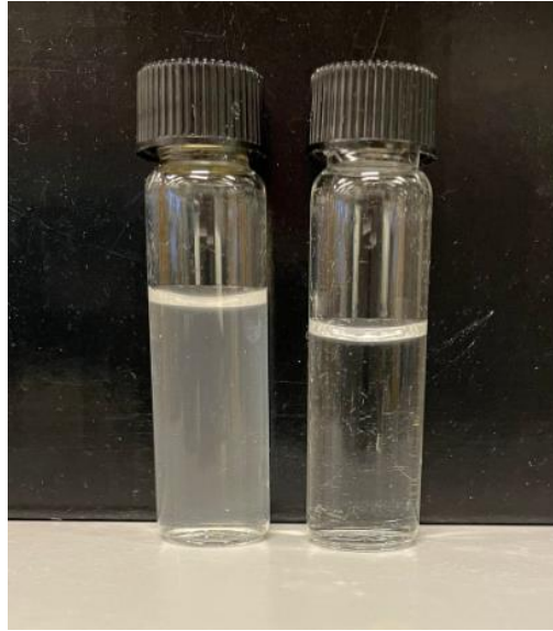
Figure 3.7 Example of produced water with \text{BaSO}_4 precipitation (left) and without \text{BaSO}_4 precipitation (right)
