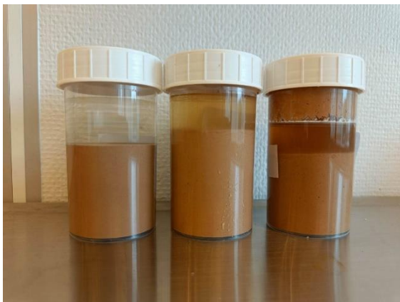
Figure 5.5: Pictures of the sample from left; reference, reference +1g chia, reference +2g chia
