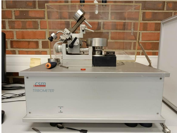
Figure 4.8: CSM tribometer instrument used for friction tests
