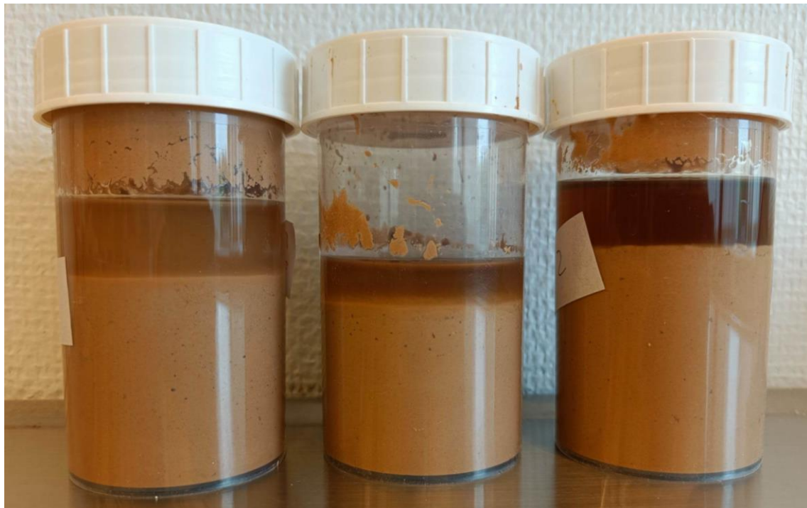
Figure 5.30: Photo of the samples from left to right; Ref, Ref+1.5g MPP, and Ref+2g MPP
