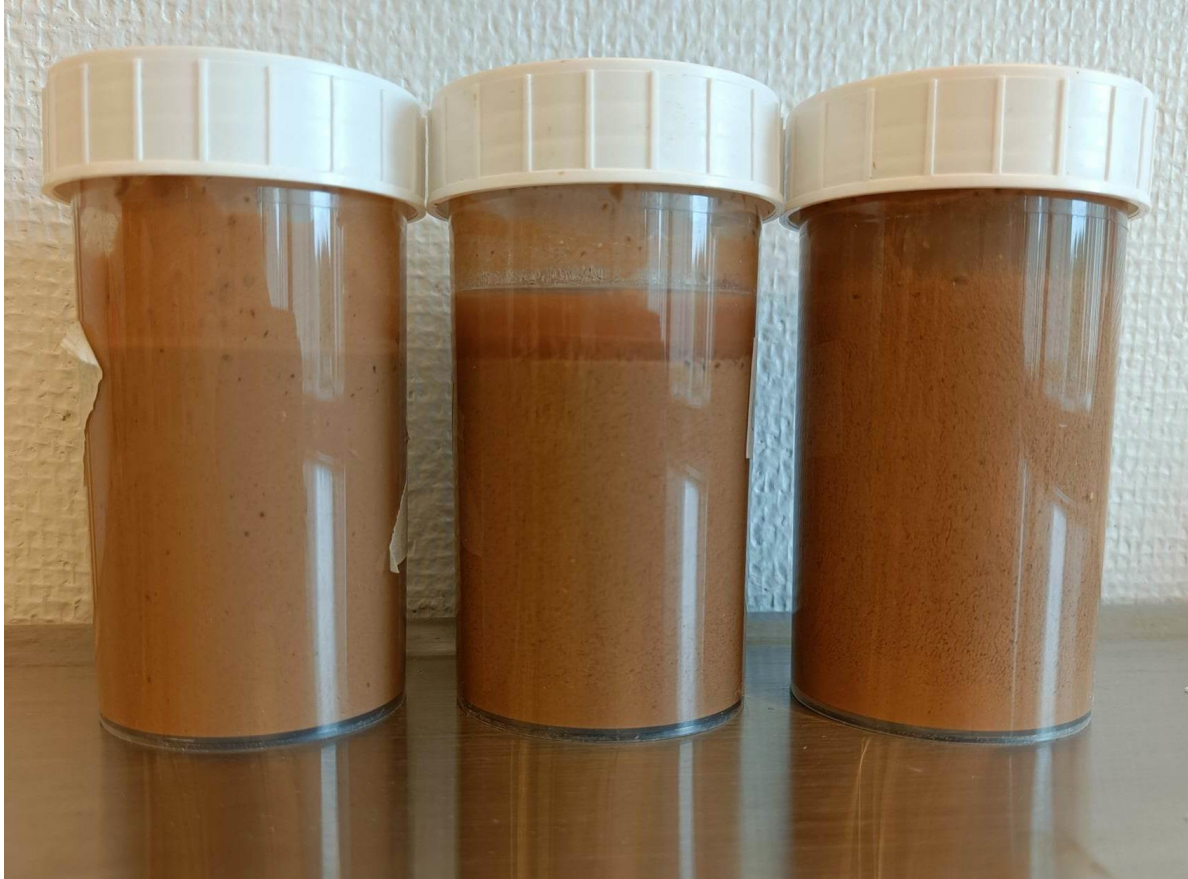
Figure 5.19: Picture containing the samples from left; KCl+2.14g XG, KCl+1.5g XG + 1g Chia, KCl+1.5g XG +2g Chia
