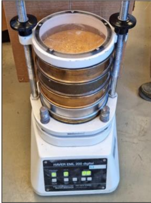
Figure 4.9: Siever shaker shaking mandarin peel powder
