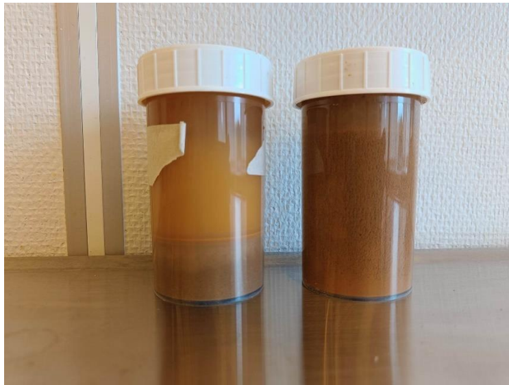
Figure 5.13: Picture of two samples containing 2g uncooked chia, the left containing Pac and PolyPac and the right containing Xanthan Gum
