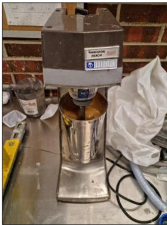
Figure 4.3: Hamilton Beach Mixer blending drilling mud
