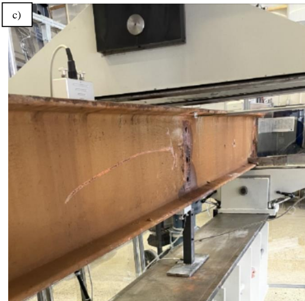
Figure 21: a) Beam setup before the buckling test, showcasing the rod for measuring lateral displacement. b) Post-test condition of the beam. c) Close-up of the beam with top and bottom strain gauges adjacent to the deflection sensor. d) The resultant damage.
