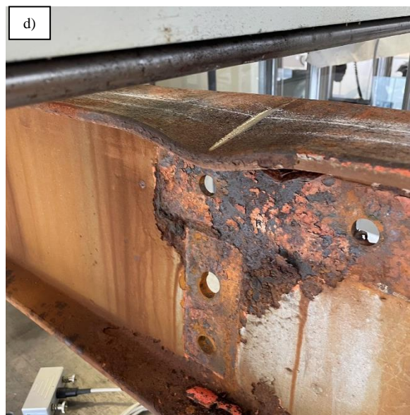
Figure 21: a) Beam setup before the buckling test, showcasing the rod for measuring lateral displacement. b) Post-test condition of the beam. c) Close-up of the beam with top and bottom strain gauges adjacent to the deflection sensor. d) The resultant damage.
