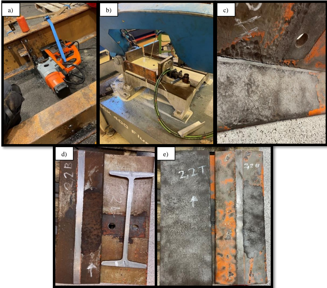
Figure 5: Procedure of dismantling and segmenting the beam for sample extraction
