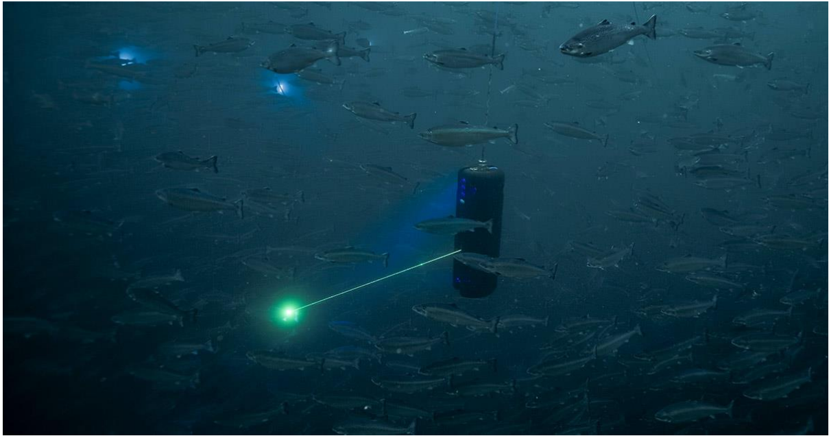
Figure 7. “The Stingray Laser System - removing salmon lice”, 2022, ( https://www.fiskerioghavbruk.no/fiskeri-og-havbruk/laser-gir-laksen-et-bedre-liv/ ) Copyright STINGRAY & MARK CABOT.
