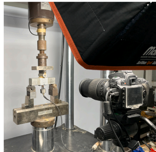
Fig. 4. The three-point bending test scheme (a), specimen geometry (b), and bending test setup (c). All dimensions in mm.
