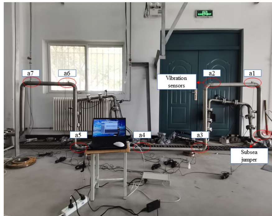
Figure 5. Slug flow-induced vibration experimental system across the jumper.
