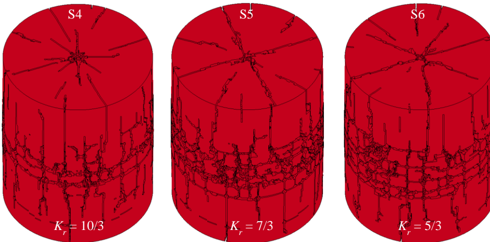
Fig. 6 Simulation results of rock blast tests (a) the final damage crack patterns, (b) crack patterns with different damage levels of test S2 and (c) fracture networks after blanking damaged rock elements ( D \leq 0.4 )
